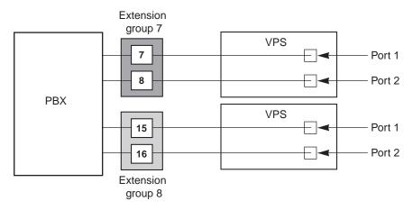
This example uses a Panasonic KX-TVS50 series VPS/KX-TVA50 series VPS, which can be connected with 4-conductor wire to 4 extension jacks of the PBX.
