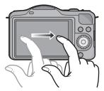
This is used to move the AF area, operate the slide bar, etc.
