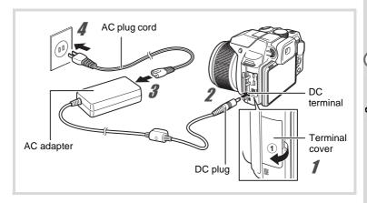
Make sure that the camera is turned off and open the terminal cover.
