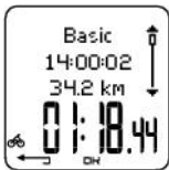
Name of exercise Time when exercise began Distance traveled Total time of exercise
