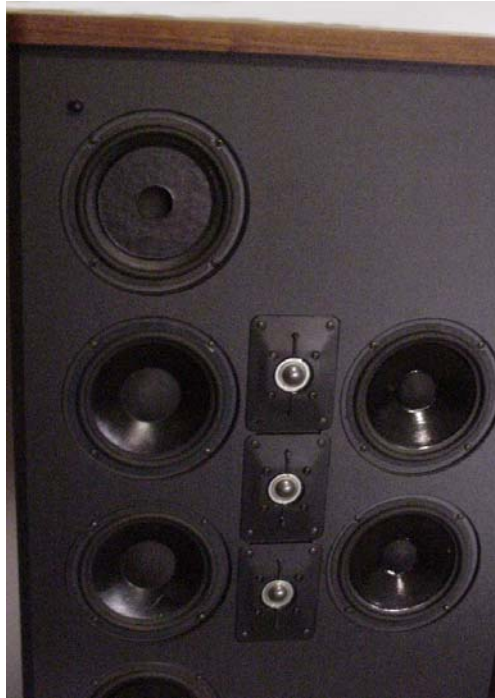
Figure 3.6. Closeup of left side SDA 2.3 showing “donut” upper stereo driver. Some of the earliest 2.3’s had stereo drivers (MW6513) with extra mass added to improve sub-bass response. Only the upper and lower driver in the four drive line source array had the donut driver.
