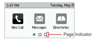
To change the displayed page, press the down or up arrow key. To change the highlighted entry, press the right or left arrow key. Press **Select** to access the desired menu.
