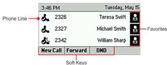
Figure 9: Phone line, favorites, and soft keys on the Lines screen on the VVX 300 series
