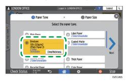
To change the envelope weight, press [ChngThickness] to specify the weight.
