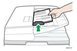
2. Place the aligned originals squarely face up in the one-pass duplex scanning ADF.
