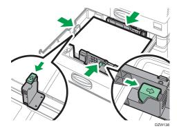
To fix the end fence, engage the two projections of the stopper with the holes on the end fence, and then tighten the fixing screw by rotating it 90 degrees clockwise with a coin or similar object.
