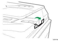
• When using the ARDF to scan originals with a paper weight less than 42 g/m<sup>2</sup> (11 lb. Bond), move the slide tray on the original output tray to the left side. When the slide tray of the Auto Reversible Document Feeder (ARDF) is in the left, the amount of output paper will be low. After scanning a thin original, return the slide tray to the previous position.
