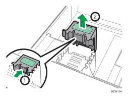
2. Put the auxiliary side fence into the groove for the paper size to use.
