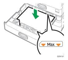
6. While pressing the release lever, adjust the side and end fences to the paper size. Do not leave spaces between the paper and fences.
