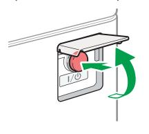
The main power indicator on the right side of the control panel turns off. The main power turns off automatically after the machine has shut down properly.
