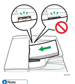
• To scan originals larger than B4 or  $8^{1}/_{2} \times 14$  size, raise the ADF's extender on the ADF output tray.
