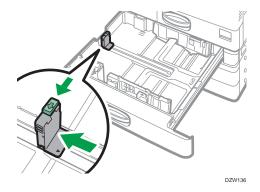
4. While pressing the release lever of the end fence, slide the end fence outward.
