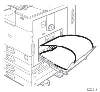
• When using paper that has a horizontal width of 457.2–900 mm (18.00–35.5 inches), set the paper so that its leading edge protrudes from the banner paper guide tray.
