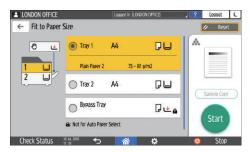
When the orientations of the original and paper in the paper tray do not match, the machine rotates the copied image automatically. To reduce an original of A3 (11 × 17) size to A4 ( $8^{1}/_{2} \times 11$ ) size, for example, you can select either A4 ( $8^{1}/_{2} \times 11$ ) $\square$  or A4 ( $8^{1}/_{2} \times 11$ ) $\square$ .
