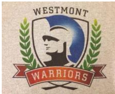
Figure 7.1-1: Image Darker Than Garment- White Ink Not Needed
