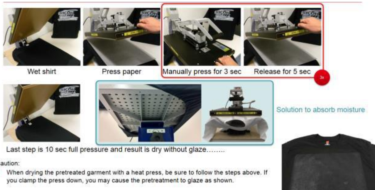
Figure 7.4-2: Heat Press Drying Procedure
