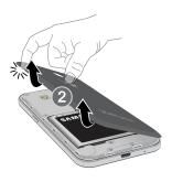
**Warning**: Do not bend or twist the back cover excessively. Doing so may damage the cover.
