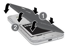
Press along the edge of the back cover until you have a secure seal.
