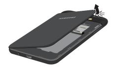
2. Lift the cover up and to the left of the device.
