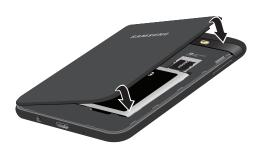
Press along the edge of the back cover until you have a secure seal.
