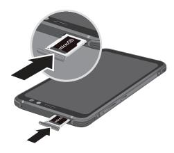
Slide the SIM card/Memory card tray back into the slot. **Note**: Your device is IP68 rated for dust and water resistance. To maintain the water-resistant and dust-resistant features of your device, make sure that the SIM card/Memory card tray openings are maintained free of dust and water, and the tray is securely inserted prior to any exposure to liquids. For more information, refer to "Maintaining Water and Dust Resistance" on page 209.
