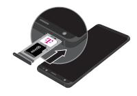
Slide the SIM card/Memory card tray back into the slot.
