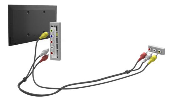
Once the connection has been made, press the **SOURCE** button to select the connected external device.
