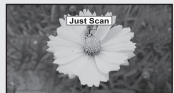
Just Scan Use the function to see the full image without any cutoff when HDMI (720p/1080i/1080p), Component (1080i/1080p) or DTV (1080i) signals are input.
