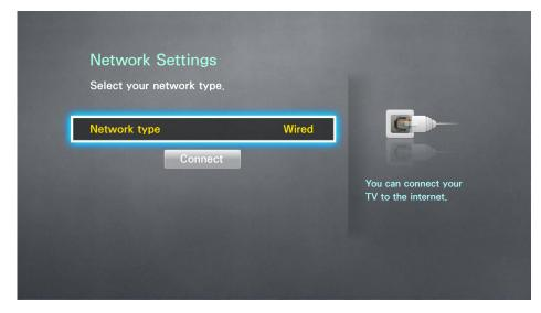
21 Select **Stop** when the TV attempts to connect to the network. Once the network connection has been interrupted, select **IP Settings**.
