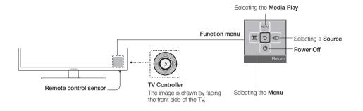
Exits the menu when pressing the controller more than 1 second. when selecting the function by moving the controller to the up/down/left/right directions, be sure not to press the controller. If you press it first, you cannot operate it to move the up/down/left/right directions.
