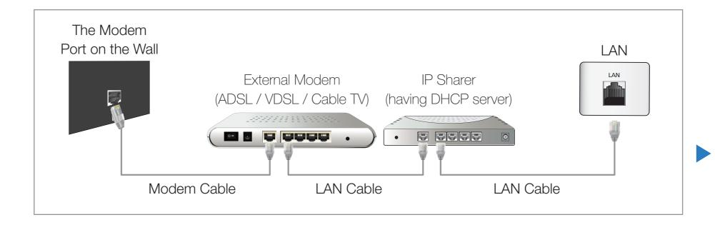
Depending on how your network is configured, you may be able to attach your TV to your LAN by connecting the LAN port on the back of your TV directly to a network wall outlet using a LAN cable. See the diagram below. Note that the wall outlet is attached to a modem or router elsewhere in your house.
