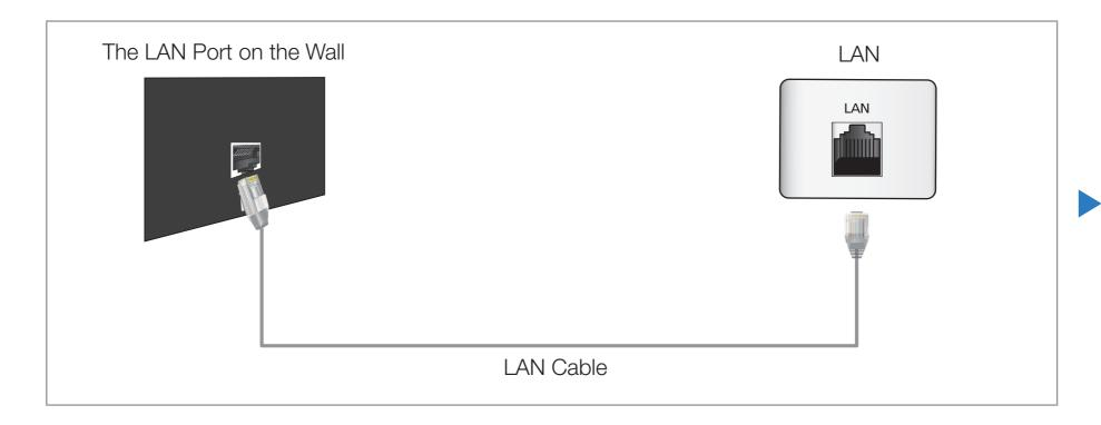
• If you have a Dynamic Network, you should use an ADSL modem or router that supports the Dynamic Host Configuration Protocol (DHCP). Modems and routers that support DHCP automatically provide the IP address, subnet mask, gateway, and DNS values your TV needs to access the Internet so you do not have to enter them manually. Most home networks are Dynamic Networks.
