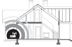
Unsuitable router position
