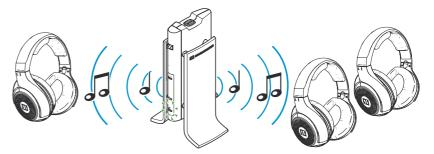
When pressing the transmitter's multi-function button 0 3 in multi-user operation, the transmitter switches to single-user operation. You can still listen to your sound source with the last headphones paired, the other headphones are disconnected from the transmitter.
