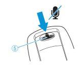
To mute the headset's microphone during a call (the LINK LED 4) on the base station lights up blue):
