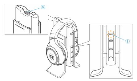
▶ Place the headphones on the headphone holder/charger of the transmitter. Make sure that the headphones make good contact with the charging contacts ⑤.
