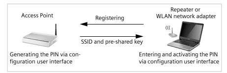
WLAN adapters without WPS can also be set up manually, i.e. the SSID and key must be entered manually. How you can find out which SSID and which pre-shared key is set, you can read in chapter "Configuring wireless connections" on page 83.
