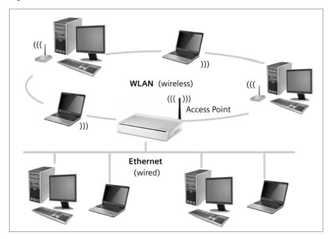
The Gigaset SX763 WLAN dsl has four Ethernet interfaces (LAN ports). Up to four PCs can be connected directly to these LAN ports.
