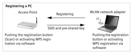
The first time this button is pressed, the device automatically creates a SSID and a pre-shared key, if these had not been already set on delivery or has been configured before manually. If a client activates WPS registration within the two-minute interval, the security data is exchanged and a connection is established. Only **one** client may synchronise during the two-minute interval. After the successful synchronization the registration is closed.
