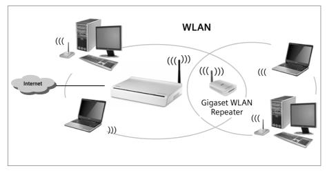
PCs to be connected in a wireless local area network via a repeater must be equipped with an integrated wireless network adapter or you have to connect an external wireless network adapter (e.g. a USB adapter).
