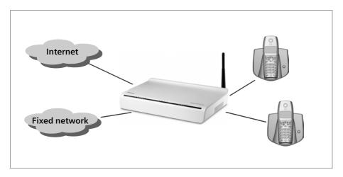
You can choose whether to connect any two analogue phones, a fax machine or an answering machine to the phone ports. You can configure these ports using the Gigaset SX763 WLAN dsl.
