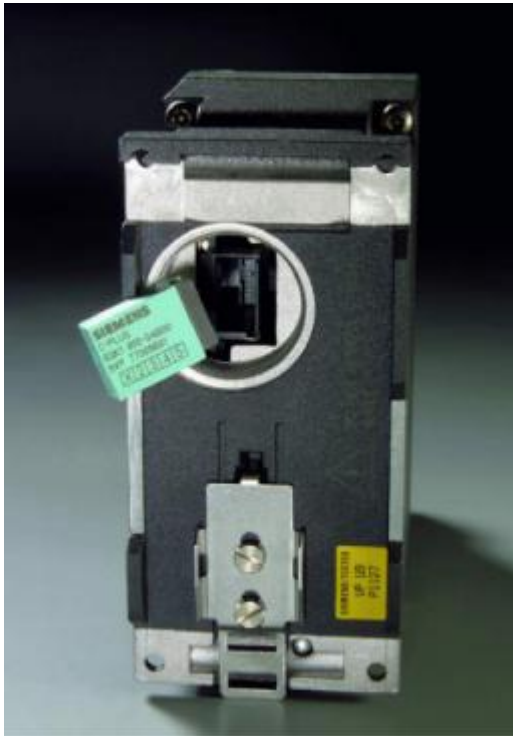
Figure 3-2 C-PLUG and slot based on the example of an X-200
