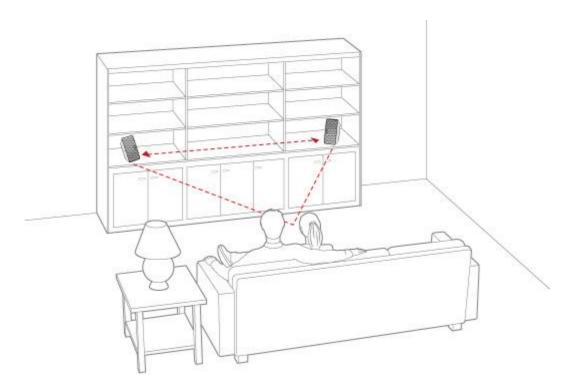
**Note:** The stereo pair setting is for use with PLAY:1, PLAY:3 and PLAY:5 units only. You cannot create a mixed stereo pair—both Sonos products in the stereo pair must be the same.
