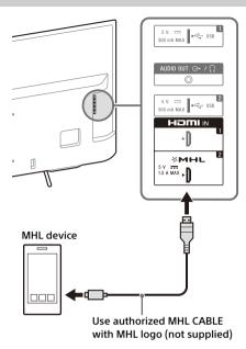
The TV simultaneously charges the MHL-compatible connected device while playing photo/music/video files. You can use the TV remote control to control the connected MHL-compatible device.
