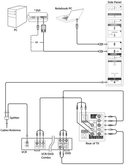
\* DVI does not support audio signals. Connect the audio output of the PC to the PC speakers or an A/V receiver to listen to sound from the PC.
