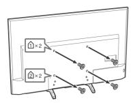
$\label{eq:decomposition} 2 \ \ \text{Attach the Wall-Mount Bracket (not supplied) using the screws (not supplied).}$
