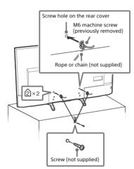
The length of the M6 machine screw differs depending on the rope or chain diameter. Please see below illustration.
