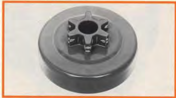
Worn chain sprocket
