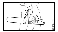
The chain guard (scabbard) should be over the chain and the guide bar, which should point backwards. When carrying your saw, the bar should be behind you.
