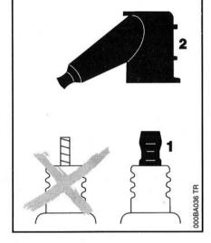
Fit a new spark plug after approx. 100 operating hours or earlier if the electrodes are badly eroded.
