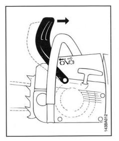
Pull the hand guard back toward the front handle: The chain brake is now disengaged - Co your saw is ready for operation.
