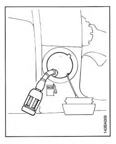
STIHL recommends the use of a suitable tool (e.g. screwdriver end of combination wrench) to tighten the cap securely. Check fuel cap periodically for tightness
