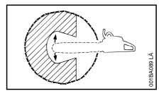
First, cut a large, wide felling notch. Make a plunge cut in the centre of the notch.
