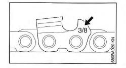
The chain pitch (e.g. 3/8) is marked on the depth gauge side of each cutter.
