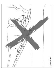
Never work on a ladder, or on any other insecure support. Never use the saw above shoulder height.
