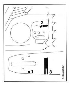
Measure groove depth with scale on filing gauge\* at nose of Duromatic bars in area used most for cutting on Rollomatic bars -
