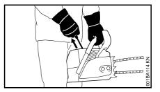
Grip the front handlebar of the saw firmly with your left hand and press down. For saws with a rear handle level with the ground, put the toe of your right foot into the rear handle and press down. With your right hand pull out the starter grip slowly until you feel a definite resistance and then give it a brisk, strong pull.
