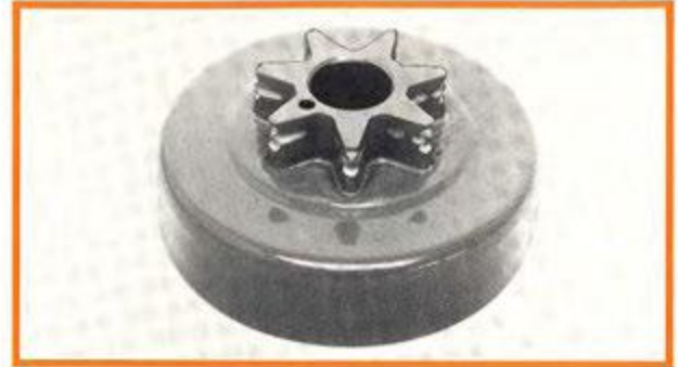
Worn chain sprocket
