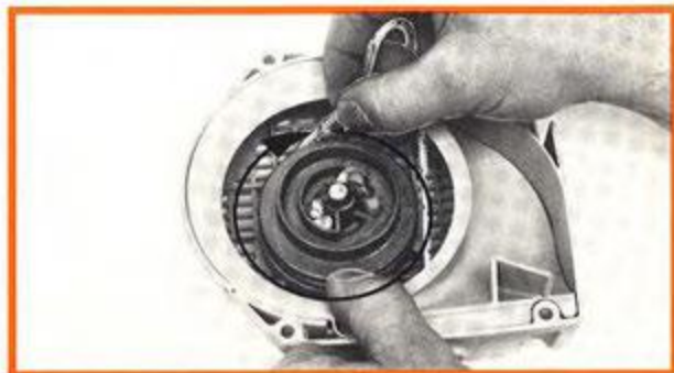
Tensioning the rewind spring
