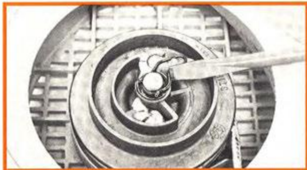
Installing the spring clip
