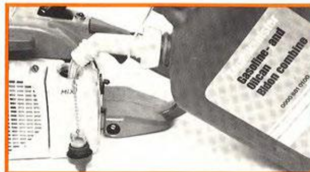
Fueling machine from gasoline and oil can
