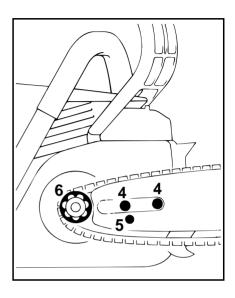
Fit the guide bar over the studs (4) cutting edges on top of bar must point to right and engage the peg
