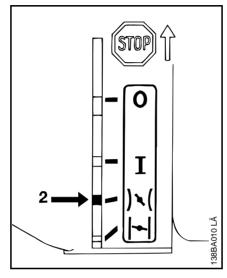
"Warm Start" position: Choke shutter is open throttle trigger is in starting-throttle position
