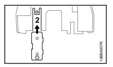
Pry the shutter (1) out of the carburator box cover (summer position) and slide it into the slot (2) (winter position)
