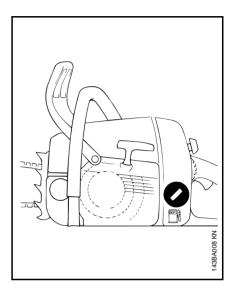
Before fueling, clean the fuel filler cap and the area around it to ensure that no dirt falls into the tank.
