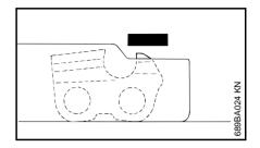
Round off depth gauges parallel to the stamped marking.
