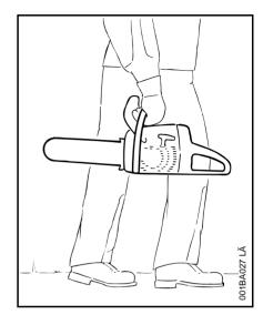
The chain guard (scabbard) should be over the chain and the guide bar, which should point backwards. When carrying your saw, the bar should be behind you.
