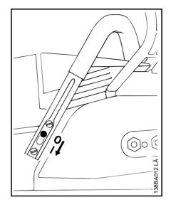
Switching on electric handle heating\*
