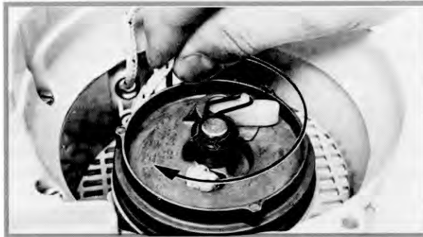
Tensioning the rewind spring
