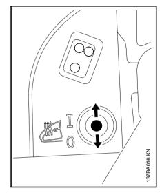
Switching on electric handle heating
