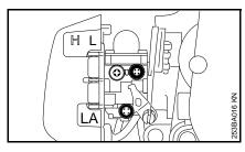
Adjust idle speed with the idle speed screw (LA) so that the cutting blades do not run
