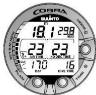
Figure 6.16. The lowest bar graph blinks to indicate that the OLF value shown relates to OTU.
