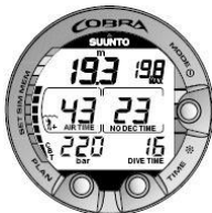
Figure 6.2. Diving display. Present depth is 19.3 m /63 ft and no decompression stop time limit is 23 minutes in A0/P1 mode. Maximum depth during this dive was 19.8 m/65 ft, elapsed dive time is 16 minutes.
