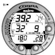
Figure 6.14. Oxygen partial pressure and OLF displays. There is an audible alarm as oxygen partial pressure is greater than 1.4 bar or set value, and/or the OLF has reached 80% limit.
