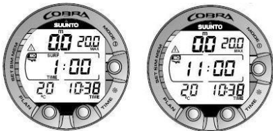
Figure 7.2. Surface interval, the surface time and no-flying time displays: Pressing the TIME button once the surface time display is shown and by pressing the TIME button twice the no-flying time display is shown, indicated by the airplane symbol.
