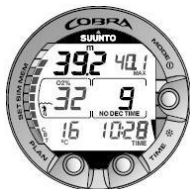
Figure 6.15. Alternative display. Pressing TIME button displays current time, maximum depth, temperature, CBT and O2%, if Air Time is less than 30 minutes.
