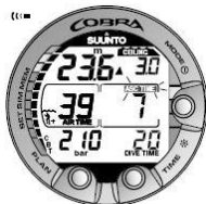
Figure 6.9. Decompression dive, below floor. Upward pointing arrow, blinking ASC TIME label and an audible alarm tell you to ascend. Minimum total ascent time including safety stop is 7 minutes. Ceiling is at 3 m/10 ft.
