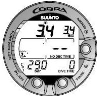
Figure 6.1. The dive has just begun and no air time is shown. First estimate of remaining air time will be shown after 30–60 seconds.
