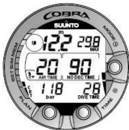
Figure 6.4. Bookmark activation. An annotation, Bookmark, is placed in the profile memory during a dive by pressing PLAN button. Note Logbook symbol.
