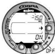
Figure 5.3. Setting Maximum Depth Alarm. Press scroll buttons to change alarm on/off and to set maximum depth value.
