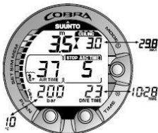
Figure 6.11. Decompression dive, at ceiling zone. Two arrows point at each other (“hour glass”). You are in the optimum ceiling zone at 3.5 m/11 ft and your minimum ascent time is 5 minutes. Pressing TIME button activates alternative display.
