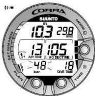
Figure 6.5. Cylinder pressure warnings. Pressure has dropped below 50 bar /725 psi. Pressure display is blinking and there is an audible alarm.
