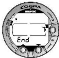
Figure 7.4. Logbook, end of the memory. END text is displayed between oldest and the most recent dive.
