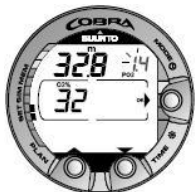
Figure 5.4. Setting Oxygen Percentage and Partial Pressure. The equivalent maximum depth is displayed as 32.8 m /107 ft. Press scroll buttons to change oxygen percentage and to set oxygen partial setting value.
