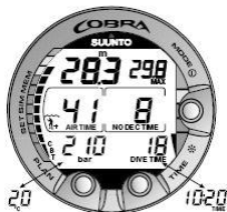
Figure 6.3. Diving display. Present cylinder pressure is 210 bar/3045 psi and remaining air time 41 minutes. Alternative display of current time and temperature is shown for 5 seconds after pressing TIME button.
