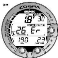
Figure 6.12. Decompression dive, above ceiling. Note a downward pointing arrow, an Er warning and an audible alarm. You should immediately (within 3 minutes) descend to or below ceiling.
