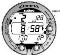
Figure 7.7. Logbook, page III. Surface interval time, average depth and consumed air indicated by \Delta P .
