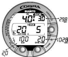
Figure 5.9. A Mandatory Safety Stop. You are advised to make a Mandatory Safety Stop in the depth zone between 6 m and 3 m/20 ft and 10 ft. Press the TIME button to view the alternative display.
