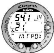
Figure 6.13. Nitrox display. Maximum depth based on set O_2\% (21%) and PO_2 (1.4 bar) is 54.1 m/177 ft.
