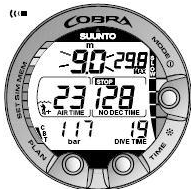
Figure 6.6. Ascent Rate Indicator. Blinking depth reading, SLOW and four segments shown: ascent rate is more than 10 m/min/33 ft/min. This is a caution to slow down! The STOP sign means that you are advised to make a Mandatory Safety Stop when you reach the depth of 6 m/20 ft.
