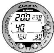
Figure 6.17. The Gauge mode. The present depth, maximum depth, dive time, cylinder pressure, remaining air time and ascent rate indicator are displayed during the dive.
