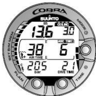
Figure 6.10. Decompression dive, above the floor. The upward pointing arrow has disappeared and the ASC TIME label has stopped blinking, which means that you are in the decompression range.
