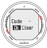
Fig. 5.28 No code stored, unit ready for pairing with transmitter
