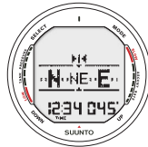
Fig. 4.2. Pressing Select (S) locks the current bearing, 45 degrees North East
