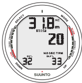
Fig. 6.18. OLF Display. Oxygen Limit Fraction (OLF) has reached 33% limit.
