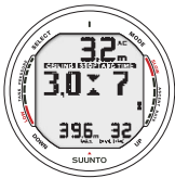
Fig. 6.12. Decompression dive, at ceiling zone. Two arrows point at each other ("hour glass"). You are in the optimum ceiling zone at 3.2 m [11 ft] and your minimum ascent time is 7 minutes..
