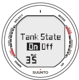
Fig. 5.24 Wireless intergartion disabled (off), press up/down to activate. Tank pressure alarm is currently set to 35bar pressure.
