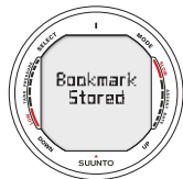
Fig. 6.3. Bookmark activation. An annotation, Bookmark, is placed in the profile memory during a dive by pressing SELECT button.
