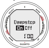
Fig. 5.20 Setting Safety/Deep stops. Press up/down buttons to change settings.
