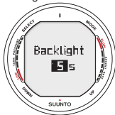
Fig. 3.15. Setting Backlight Time. Press up/down to change backlight on/off and to set time value.
