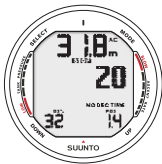
Fig. 6.17. PO 2 Display. Oxygen Partial Pressure is 1.4 bar
