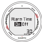
Fig. 5.11. Setting Dive Time Alarm. Press up/down buttons to change alarm on/off and to set dive time value. Press Select to accept/move to next setting.
