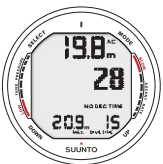
Fig. 6.2. Diving display. Present depth is 19.8 m [66 ft] and no-decompression stop time limit is 28 minutes. Maximum depth during this dive was 20.9 m [70 ft], elapsed dive time is 15 minutes.
