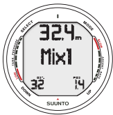
Fig. 5.13. Setting primary gas mix (MIX1). Oxygen percentage is 32%, oxygen partial pressure limit is 1.4 bar. The equivalent maximum depth is displayed as 32.4 m [106 ft]. Press scroll buttons to change oxygen percentage and to set oxygen partial setting value. Accept settings by pressing SELECT.
