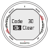
Fig. 5.29 Unit is paired on channel 32. Select Clear to erase code, OK to accept.
