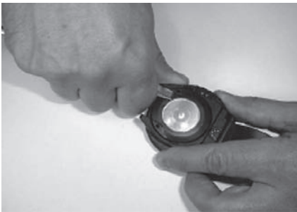
Fig. 5.2 Opening of the securing ring.
