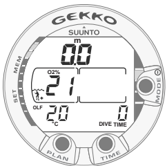
Fig. 3.21. Surface display in the Nitrox mode
