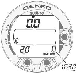
Fig 3.3. Startup III. Surface mode. Depth and dive time are zero, current temperature, 20 °C. Pressing TIME button activates alternative display of current time.
