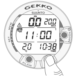
Fig. 3.28. Surface interval, no-flying time. Pressing TIME button twice will show no-flying time, indicated by an airplane symbol.
