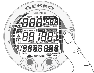
Fig. 3.1. Startup I. All segments shown.
