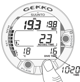
Fig. 3.7. Diving display. Present depth is 19.3 m [63 ft] and no-decompression stop time limit is 23 minutes in A0/P1 mode. Maximum depth during this dive was 19.8 m [65 ft], water temperature is 18°C [64°F], elapsed dive time is 16 minutes. Alternative display of current time 10:20 [10:20 am] is shown for 5 seconds after pressing TIME button.
