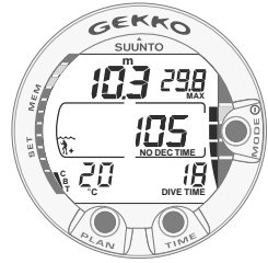
Fig. 3.11. Ascent Rate Indicator. Maximum allowed ascent rate. Four segments
