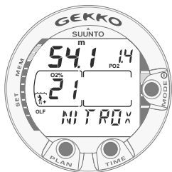
Fig. 3.20. Nitrox display. Maximum depth based on set O 2 % (21%) and PO 2 (1.4 bar) is 54.1 m [177 ft].
