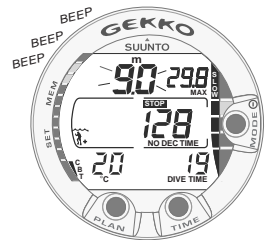
Fig. 3.12. Ascent Rate Indicator. Blinking depth reading, SLOW and four segments are shown together with an audible alarm: ascent rate is more than 10 m/min [33 ft/min]. This is a caution to slow down! STOP sign means that you are advised to make a Mandatory Safety Stop when you reach a depth of 6 m [20 ft].
