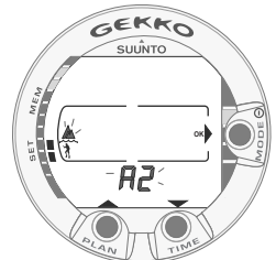
Fig. 4.25. Setting Altitude adjustment. Press scroll buttons to change altitude mode.
