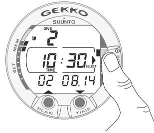
Fig. 4.10. Logbook, page I. Press SMART (Select) button once to be able to scroll between different dives.
