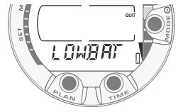
Fig. 3.2. Startup II. Battery power indicator.
