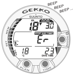
Fig. 3.18. Decompression dive, above ceiling. Note downward pointing arrow, Er warning and an audible alarm. You should immediately (within 3 minutes) descend to or below ceiling.
