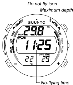
Fig 4.24 Surface interval, display II. The desaturation time/no-flying time, indicated by an airplane symbol, is 11 h 25 min. The maximum depth of the dive was 29.8 m [98 ft].
