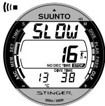
Fig. 3.15 Ascent Rate Indicator. Blinking SLOW and four segments are shown together with an audible alarm: ascent rate is more than 10 m/min [33 ft/min]. This is a caution to slow down! STOP sign means that you are advised to make a Mandatory Safety Stop when you reach a depth of 6 m [20 ft].
