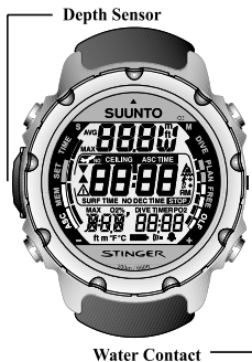
Fig. 2.2. The water contact and depth sensor.
