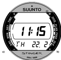
Fig. 2.5. The time keeping display a) the date is displayed b) the seconds are displayed c) the dual time is displayed.
