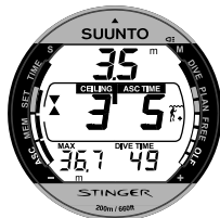
Fig. 3.19. Decompression dive, at ceiling zone. Two arrows point at each other ("hour glass"). You are in the optimum ceiling zone at 3.5 m [11 ft] and your minimum ascent time is 5 minutes.
