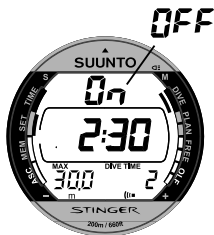
Fig. 4.13. Dive Time Alarm. Center window displays less than 5 minutes dive time.
