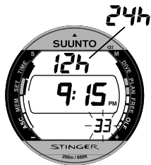
Fig. 4.3. The Time Adjustment Mode is activated and the second digits are blinking. Page I.
