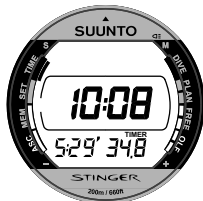
Fig. 2.7. The Stopwatch displays hours, minutes and seconds.
