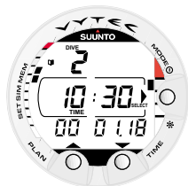
Fig. 4.11. Logbook, page I. Press SMART (Select) button once to be able to scroll between different dives.
