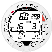
Fig. 3.11. A three minute Recommended Safety Stop.
