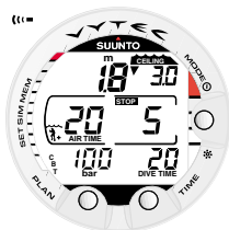
Fig. 3.15. Violated Mandatory Safety Stop. Downward pointing arrow and an audible alarm indicate you should descend to ceiling zone.
