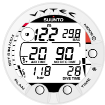
Fig. 3.10. Bookmark activation. An annotation, Bookmark, is placed in the profile memory during a dive by pressing PLAN button. Note the Logbook symbol.
