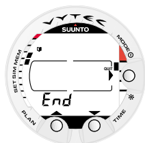
Fig. 4.12. Logbook, end of the memory. END text is displayed between oldest and the most recent dive.
