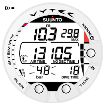
Fig. 3.12. Cylinder pressure warnings. Pressure has dropped below 50 bar [725 psi]. Pressure display is blinking and there is an audible alarm.
