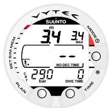
Fig. 3.7. Dive has just begun and no air time is shown. First estimate of remaining air time will be shown after 30-60 seconds.
