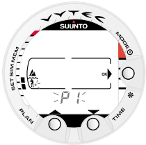
Fig. 4.24. Setting Personal adjustment. Press scroll buttons to change personal mode.
