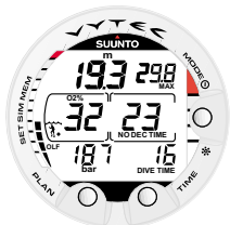
Fig. 3.22. Diving in Nitrox mode. The O 2 % is set to 32%.
