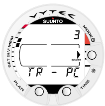
Fig. 4.15. Data Transfer mode. [3 TR-PC].
