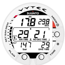
Fig. 3.23. Diving in Nitrox mode. After air time is less than 30 minutes O 2 % is substituted by Air Time display.
