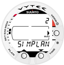
Fig. 4.19. Dive Planning Simulator mode. [2 SIMPLAN].
