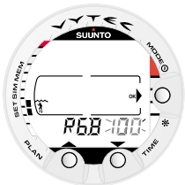
Fig. 4.25 Setting RGBM adjustment. Press scroll buttons to change setting.
