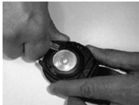
Fig. 5.2. Opening of the securing ring.
