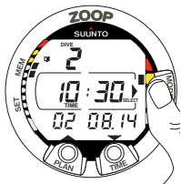
Fig. 4.10. Logbook, page I. Press SMART (Select) button once to be able to scroll between different dives.
