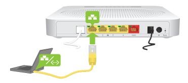
2 Connect the other end of the Ethernet cable to your network device.
