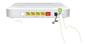
4 The ① LED turns on. Wait at least two minutes to allow your TG589vac v2 to complete the startup phase.
