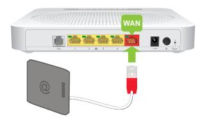
**3** Plug the other end of the cable into the Ethernet port of your Internet access device (for example, an Optical Network Terminal (ONT) for Fiber).
