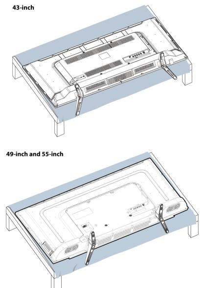
2 If the stands are installed, remove the two screws that secure each stand to your TV, then remove the stands.
