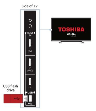
1 Plug a USB flash drive into the **USB** port on the side of your TV.
