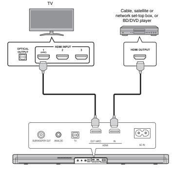
When a TV that supports Audio Return Channel (ARC) will be connected, the sound bar can only play audio from the TV when it is connected as shown above.
