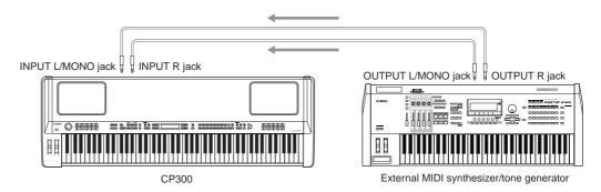
The sound of an instrument connected to these INPUT jacks cannot be adjusted from the CP300. Any level adjustments must be done from the instrument itself.
