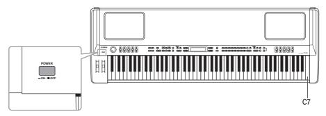
If you wish to erase Memory files at this time, simultaneously hold down the rightmost white key (C7) and black key ( $B \triangleright 6$ ) together and press the [POWER] switch to turn on the power to the CP300.
