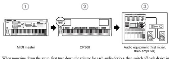
When powering down the setup, first turn down the volume for each audio devices, then switch off each device in the reverse order (first audio devices, then MIDI).
