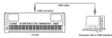
When the USB connector is connected, the MIDI connectors cannot be used.
