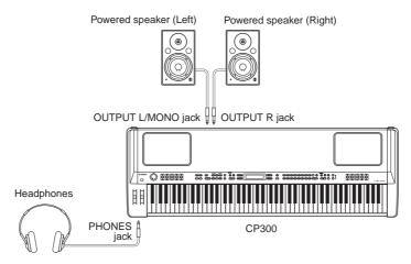
ENOTE When using just one powered speaker, connect it to the OUTPUT L/MONO jack on the rear panel.
