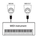
Use the [MIDI] terminals and standard MIDI cables to connect external MIDI devices (keyboard, sequencer, etc.).
