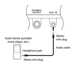
By connecting an audio device such as a portable music player to the instrument's [AUX IN] jack, you can output the sound of the audio device through the built-in speakers of this instrument. This lets you play the instrument along with the playback of your audio player.
