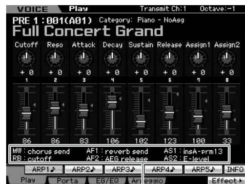
Indicates the controller assignment
