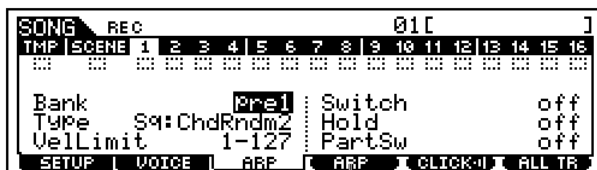
Determines whether Arpeggio playback data is recorded to the track or not. (Press the [F4] button.)
