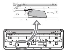
3 Insert the six new batteries, being careful to follow the polarity markings on the inside of the compartment.
