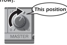
While playing your instrument or singing into the microphone, adjust the LEVEL control of the corresponding channel.
